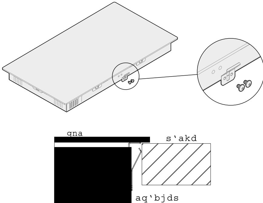
**⚠** Under any circumstances, the brackets cannot touch with the inner surfaces of the worktop after installation (see picture).
